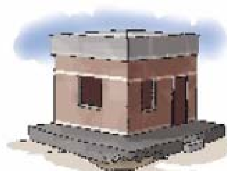
Extended plinth around the building protects from scouring
